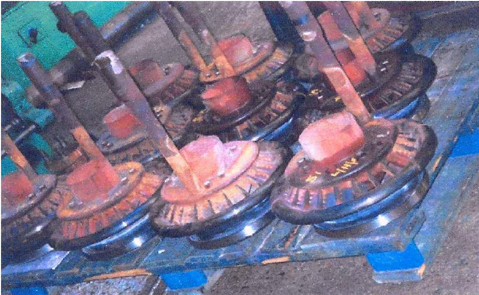
Fig 4. Recovery of location diameter on pre-mix nozzles.
