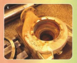
1-2. Hastelloy pump casing with location spigot and gasket face eroded and corroded by the chemical being pumped. Spiral Weld repaired using Hastelloy alloys to recover the wom location spigot and gasket face.
