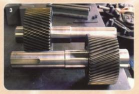
3. Typical gear wheels have had worn bearing diameters recovered either side of the gear hubs.
