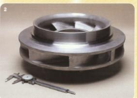
shows impeller following full recovery to as new condition.
