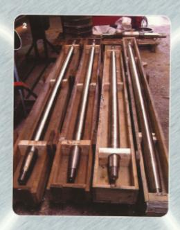
Prop shafts awaiting despatch following recovery of worn bearing and gland areas. We have extensive expertise in recovering carbon steels and more exotic materials such as Monel and Aquamet 22. Dissimilar overlays for improved performance are often used for the recovery using materials such as Inconel 625, Nitronic 50 and cobalt based alloys.
