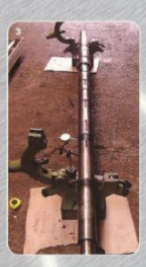
3-4. Start Standby boiler feed pump shaft undergoing initial inspection to damaged impeller location diameters and lip seal areas prior to Spiral Weld repair.
