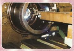
1-2. Recovery of an internal location diameter on a damaged valve head. Our low heat input process allows us to recover components with the minimum of distortion to surrounding features.
