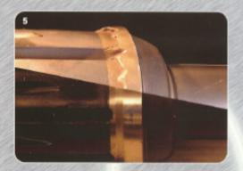
Control valve spindle showing eroded seat area in top half of picture and recovered seat in the bottom half. The seat was recovered with a cobalt based alloy to give the seat better wear resistance compared to the original design in parent material.
