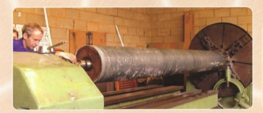
Process roller from a paper mill having the damaged bearing areas recovered at either end of the roller.
